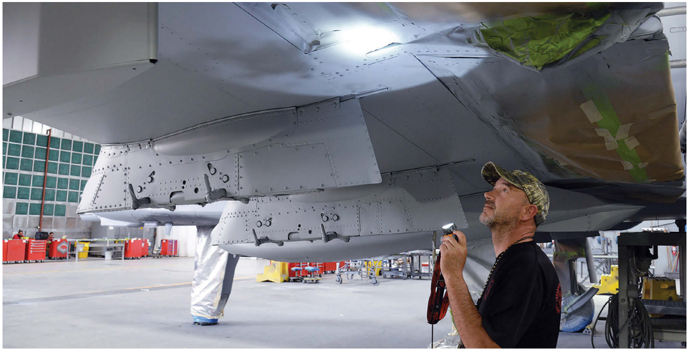
Contractor Dale Benoit inspects paint beneath a new A-10 Thunderbolt wing at Hill AFB, Utah. The aircraft was the last of 173 to receive new wings under the initial program, which extends the life of the fleet.
